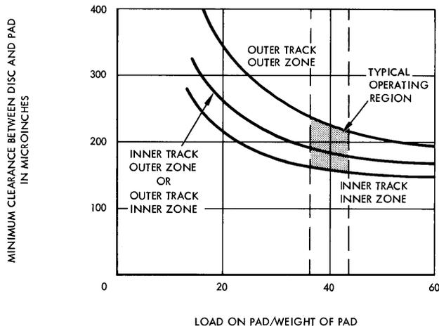
FIGURE IV THE CHARACTERISTICS OF THE HEAD PAD
