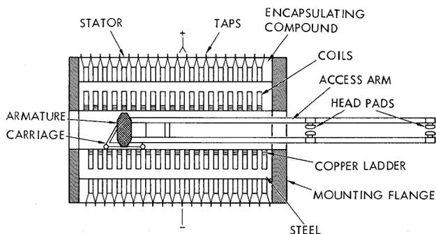
FIGURE V THE DIGITAL POSITIONER
