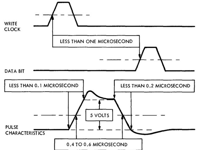
FIGURE XVI CLOCK AND DATA CHARACTERISTICS
